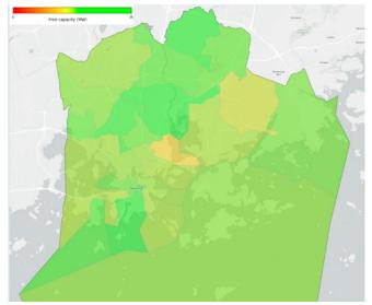
Figure 20. Free distribution network capacity for each primary substation feed area.
