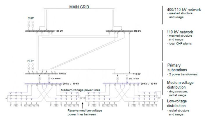
Figure 15. Basic structure of Helsinki's electricity distribution network.
